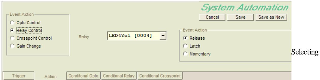
Relay Control in the Event Action Box allows you to Latch, momentarily close (~500msec), or release a (latched) relay when the event's trigger occurs.
