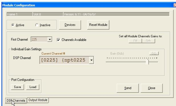
For Output cards, click on the DSP Channels Tab in the lower left corner to find the Port Configuration Save button.
