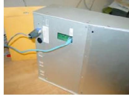
Power connection to Rubicon8 console (also note the RS485 connection via patch cable)
