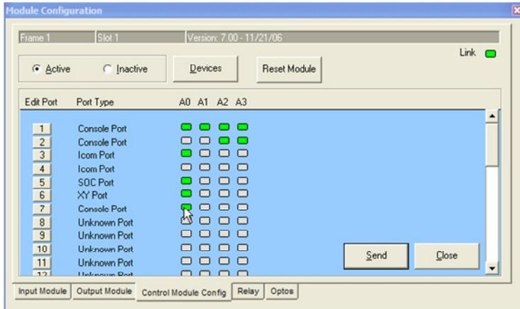
You should now see a Green dot for any active addresses on the RS-485 port. Click on the rectangle port number again to go back to RS-485 Module Configuration.
