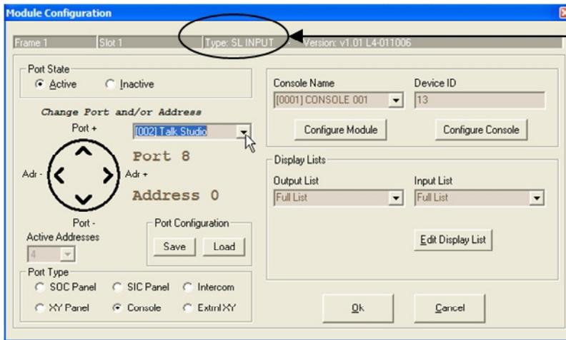
The module type should show up as an SL INPUT. Note the Port and Address control. If you have more than one TP-L4 connected to this RS485 port, you can toggle between them using the Adr+ and Adr- (left and right) arrows. If you want to configure modules on other physical RS485 ports (for the same RIO or DRC), you can change ports with the Port + and Port - (Up and Down) arrows.
