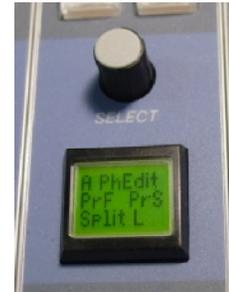
While in Edit mode the screen will have an orange backlight. Turn the Select Knob to choose how you want this module's sources to feed the Phone Editor bus. OFF means the source will feed the Phone Editor bus in normal stereo. L or R will sum the source's left and right channels and feed the sum to just the selected channel of the Phone Editor bus. When you've made your selection, press the display to save the selection.
