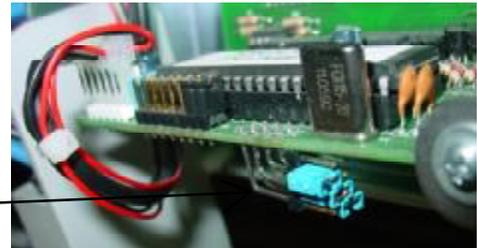
IMPORTANT NOTE: If feeding unbalanced (ESE) clock sync to the clock, use shield and the black wire - (minus) input. For more options, see the full Torpey clock manual supplied on the SAS CD that ships with the system.
