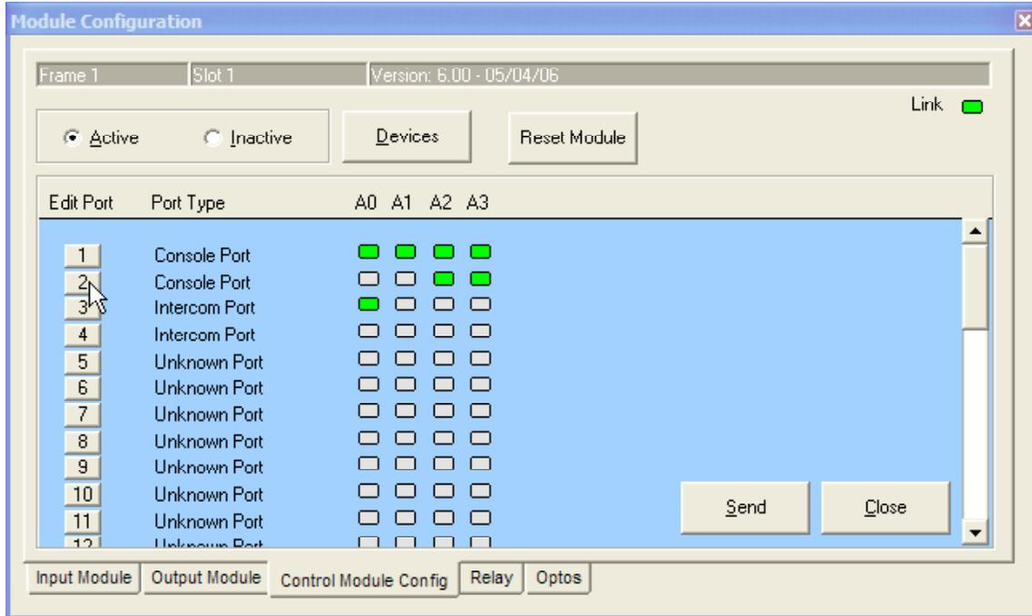
This RIO/KRL shows an eight slot console being run from the first two RS485 ports and an intercom panel connected to the third. You can see that there are active modules in the first four slots of the console, followed by two slots with nothing connected, ending with modules in the last two slots. In most cases the Control Room Monitor Module and the Console Control Module are the last two active slots.
