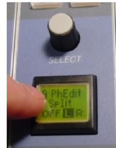
Saving the Split options will bring up the Fader option window. Turn the Select Knob to highlight either Pre or Post. Press the display to save the selection. This will bring up the Switch option window. Again, turn the Select Knob to highlight Pre or Post, then press the display to save your selection. This will cycle you back to the Split option window, which you've already set. Press the Select Knob to exit Edit mode.
