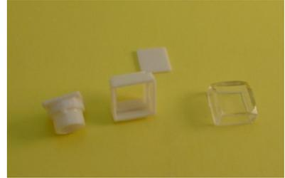
Assembly base, lens base, white diffuser, and lens.
