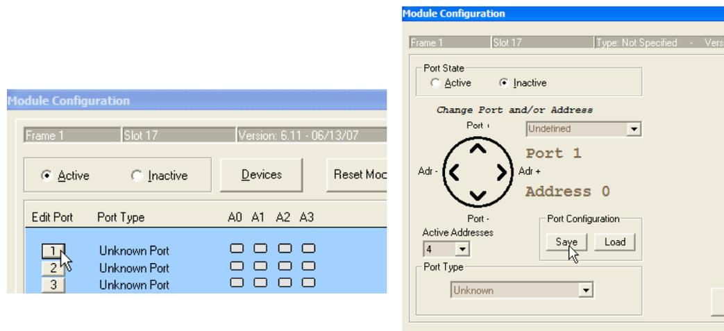
Click one of the numbered ports. Then click on the Save Port Configuration button. The filename will be Module0117.cfg if the module is in slot 17 of frame 1. Leave this filename as it is and click Save. The file contains settings for all sixteen rs485 ports on the card.
