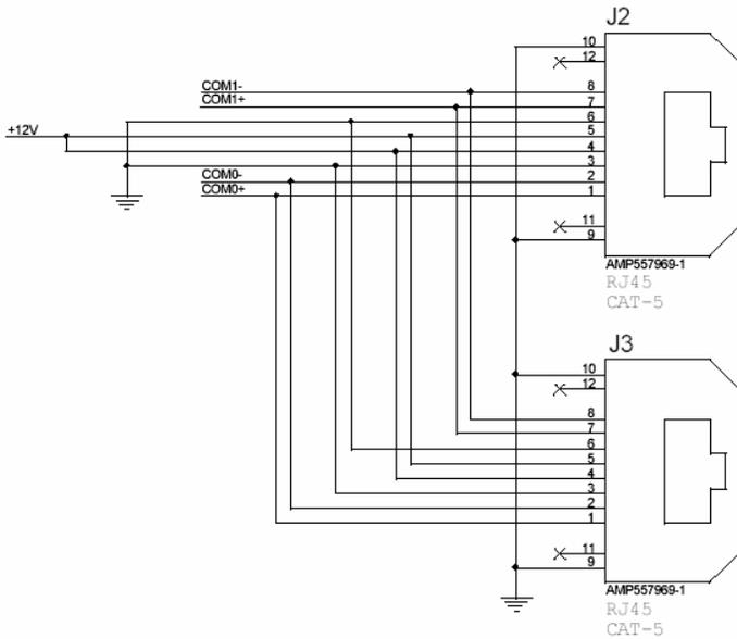
+12 volts DC and Power ground is always present at J2 & J3 (pins 3-6), even if J4 is used to supply the power.
